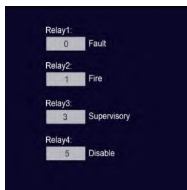
Figure 77: 1 Relay Output Setup
