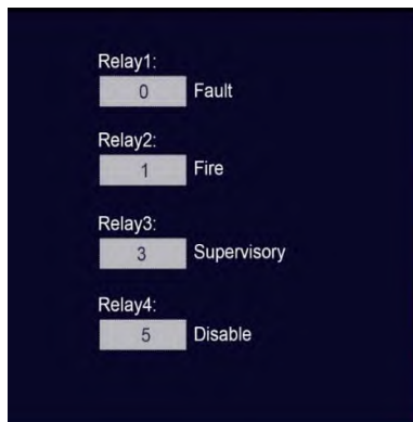
Figure 72: 1 Relay Output Setup
